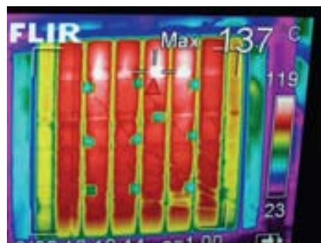
Thermal imaging of TimberStrand® LSL 2x6 studs resisting heat (yellow is cooler than red) during a fire test of the assembly.
